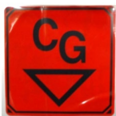
Picture 4. Sign on the frame of the milk tank, showing the centre of gravity.
